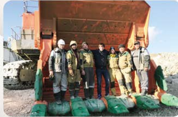
FRONT SHOVEL FOR HITACHI EX3600 EXCAVATOR BUCKET CAPACITY – 21m 3
