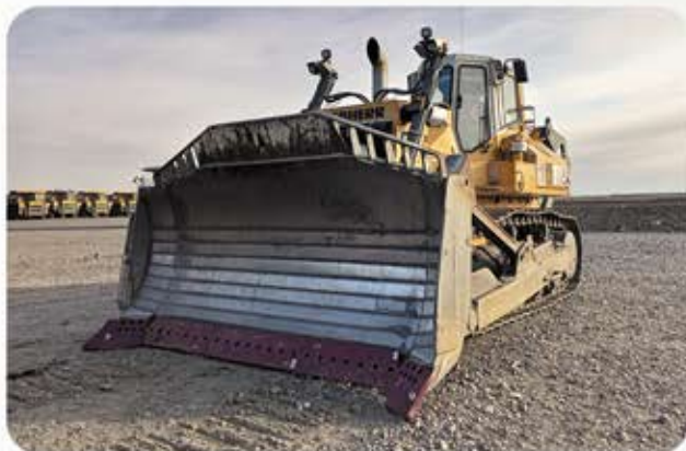
HEMISPHERICAL BLADE FOR LIEBHERR 784 DOZER BUCKET CAPACITY – 13.7m 3
